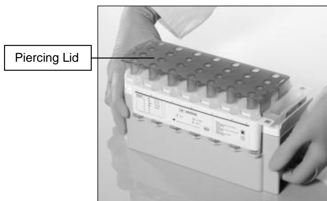
Figure 4: Piercing lid being positioned onto the reagent cartridge holder
